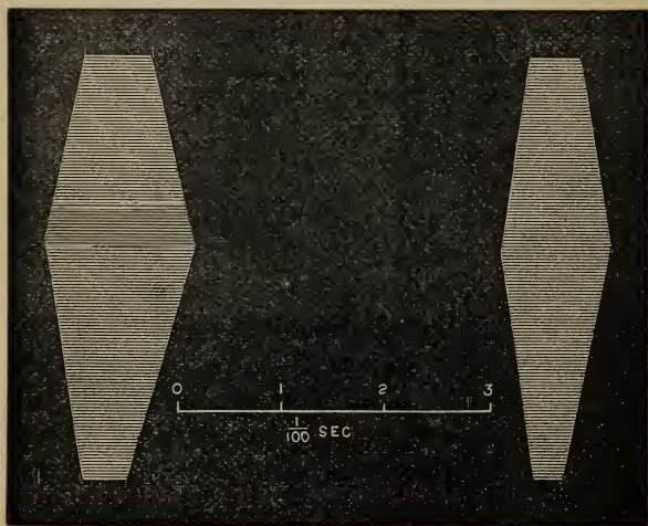
Thornton and Pickard's shutter. Diagrams taken with slit in the aperture of the shutter.
